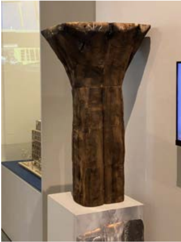
A charred remnant from a controlled burn during fire performance testing for Ascent. Photo © Joann Gonchar, FAIA
